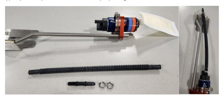
4 – Included with the install kit is a 48" (575mm) long pump harness, separate the top and bottom halves and install the pump section onto the DW420 lift pump.
