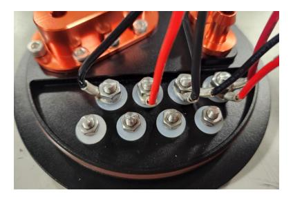
12 – Locate the four-wire pigtail harness for the fuel level, fuel temperature and low fuel light sensors. Attach this harness to the four smaller M4 terminals. Not all Silvia/Skyline applications will use all four wires, you may de-pin and remove the unused wires for a cleaner install.
