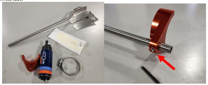
2 – Install the included rectangular prefilter sock onto the pump and clamp it to the pump holder with the worm drive hose clamp. The bottom of the pump should be approximately 1.5" (38mm) from the pump holder (not including the filter sock).
