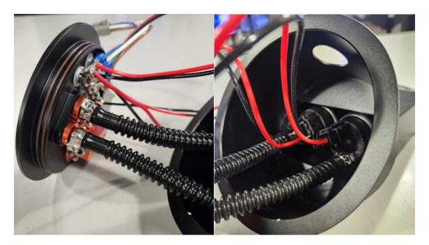
14 – Slide the two-wire lift pump harness and four wire level sensor harness through the hole in the surge tank. Lubricate the X2 module tophat with the supplied PTFE grease and install the tophat into the surge tank, this can be rotated to ease installation and, once inside the tank rotated for better fitting and wiring alignment.
