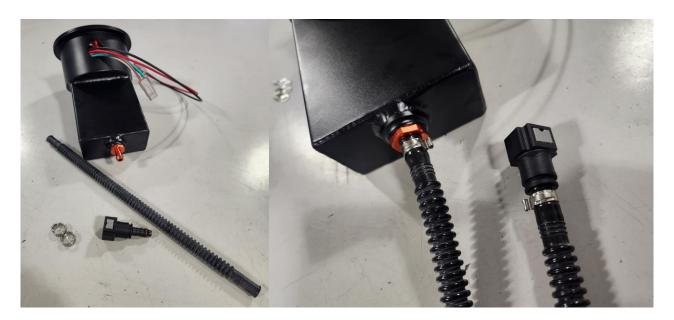
16 – Install the supplied butt connectors onto the fuel tank sensor harness wiring. These connectors feature a fuel safe heat shrink outer covering.
