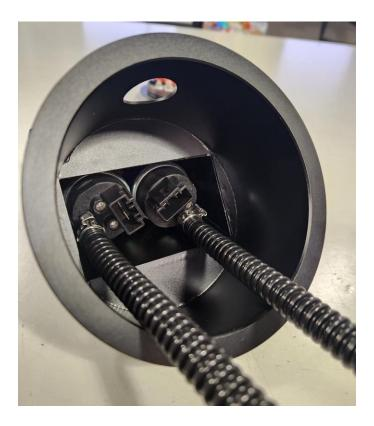
10 – Locate the upper half of the lift pump wiring harness from Step 4, the two standard pump pigtails and the six 16-14awg ring terminals. Strip and crimp the ring terminals to all three pump harnesses.
