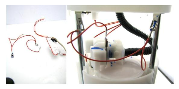
4 – push the top down and remove the c-clip from the upright and pull the top up
