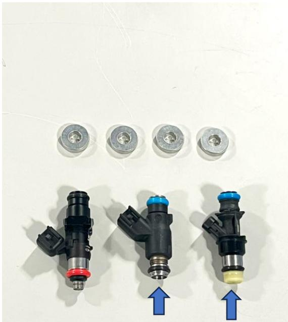
Factory LM7, LQ9, L92 Truck Injector examples next to the “Mid” height Injector from this kit.
