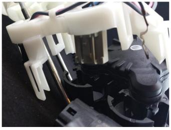
4 – remove the OE pump outlet spacers to be reused on the outlet of the DW300c/430c pumps. The OE fuel sock can be reused, but will require trimming to fit the DW300c/430c pumps
