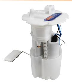
The DeatschWerks DW400 Performance Module for Nissan 350Z is now available for 2003-2009 applications. Featuring the DW400 pump, this module includes integration of the OEM returnless fuel line and retention of ALL the functionality of the factory module. The module consists of a top-hat, center section, and lower bucket. These components work together to deliver the flow you need and the OEM functionality you want.
