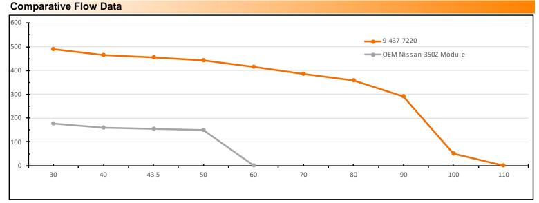
Note: All Horsepower, flow and amperage ratings tested at 13.5v and 10awg wiring.
