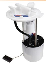
The DeatschWerks F-150 DW400 Performance Module is now available for 2015-2024 applications. Featuring the DW400 pump, this module includes integration of the OEM returnless fuel line and retention of ALL the functionality of the factory module. The module consists of a top-hat, center section, and lower bucket. These components work together to deliver the flow you need and the OEM functionality you want.
