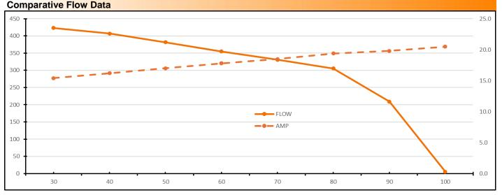
Note: All Horsepower, flow and amperage ratings tested at 13.5v and 10awg wiring.
