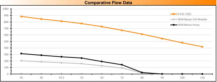
Note: All Horsepower, flow and amperage ratings tested with DW420 fuel pumps at 13.5v and 10awg wiring.
