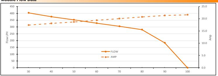
Note: All Horsepower, flow and amperage ratings tested at 13.5v and 10awg wiring.
