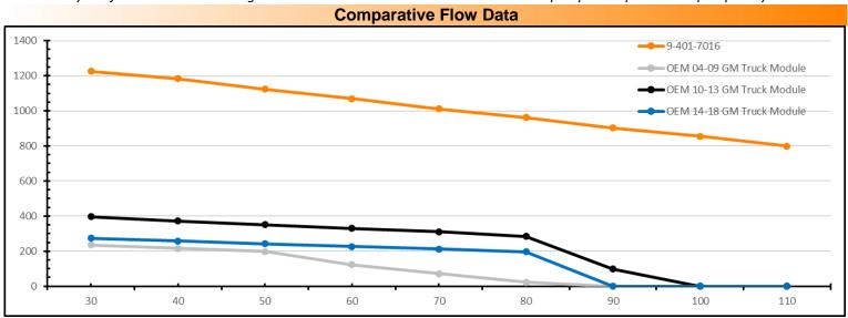
Note: All Horsepower, flow and amperage ratings tested with triple DW400 fuel pumps at 13.5v and 10awg wiring.
