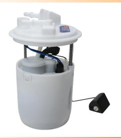
The DeatschWerks DW300 WRX Fuel Pump Module is now available for 2015-2021 applications. Featuring the DW300 pump, this module includes integration of the OEM returnless fuel line and retention of ALL the functionality of the factory module. The module consists of a top-hat, center section, and lower bucket. These components work together to deliver the flow you need and the OEM functionality you want.
