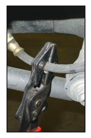
Figure 1: Hose crimper applied to OE brake hose
