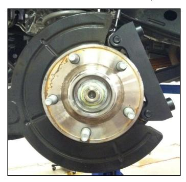
Figure 3: Front view of bracket install
