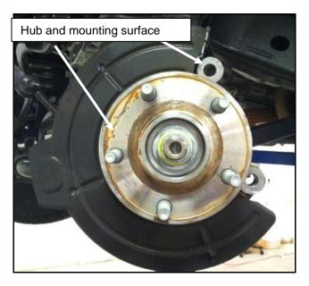
Figure 2: Rotor and caliper removed from spindle
