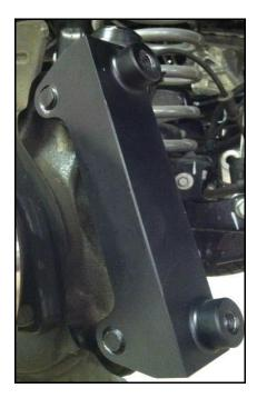
Figure 4: Intermediate bracket
