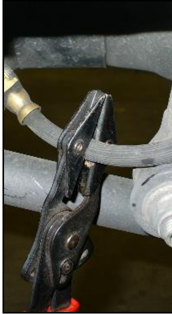
Figure 1: Hose crimpers applied to brake hose
