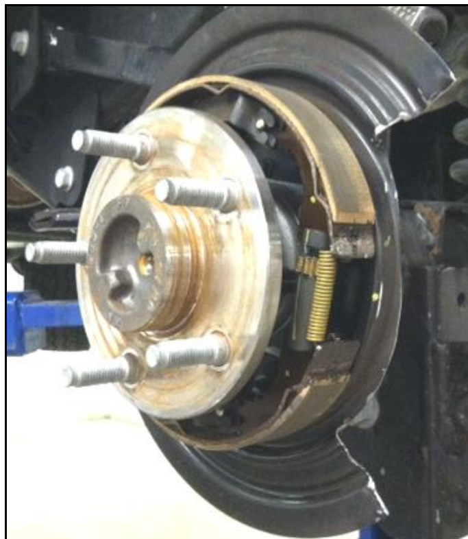
Figure 3: ¾ view of the dust shield after trimming for caliper clearance
