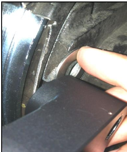
Figure 7: Shim placement between the caliper bracket and axle housing end
