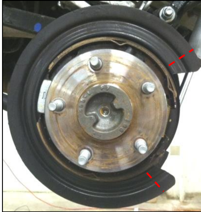
Figure 2: Outboard view of dust shield before trimming.
