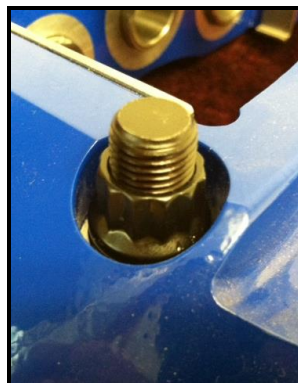
Figure 8: ARP studs, washers, and nuts installed
