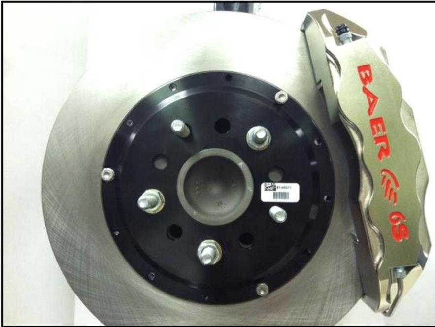
**\*\*Note:** Check for adequate clearance between the rotor and the lower control arm just below the ball joint. Due to production tolerances at the weld on the A-arm, our rotor may contact the lip at the nose. This will usually only happen when the suspension is loaded (normal ride height). A small lip is stamped into the control arm and will need to be removed for clearance. Remove the lip about 1" from each side of center and recheck for clearance.
