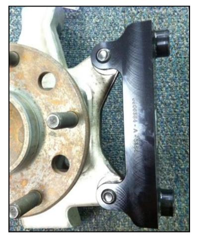
Figure 1: Base bracket installed onto spindle
