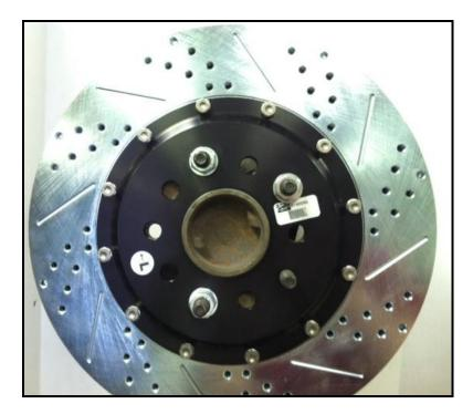
Figure 2: New rotor installed onto hub
