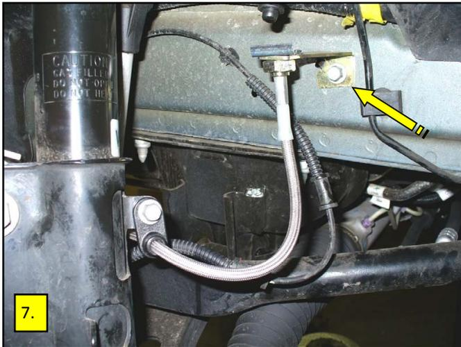
7. This picture shows the location of the hose bracket installed on the frame, ready to attach the hardline. Always double check the hose location for interference with suspension or steering components.
