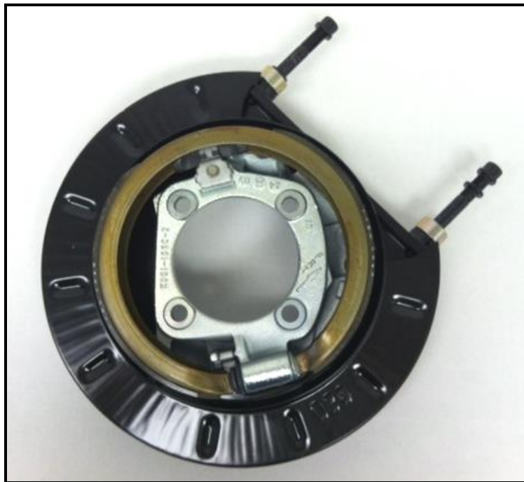
Figure 7: Outboard view of park brake assembly (spacers installed over studs)
