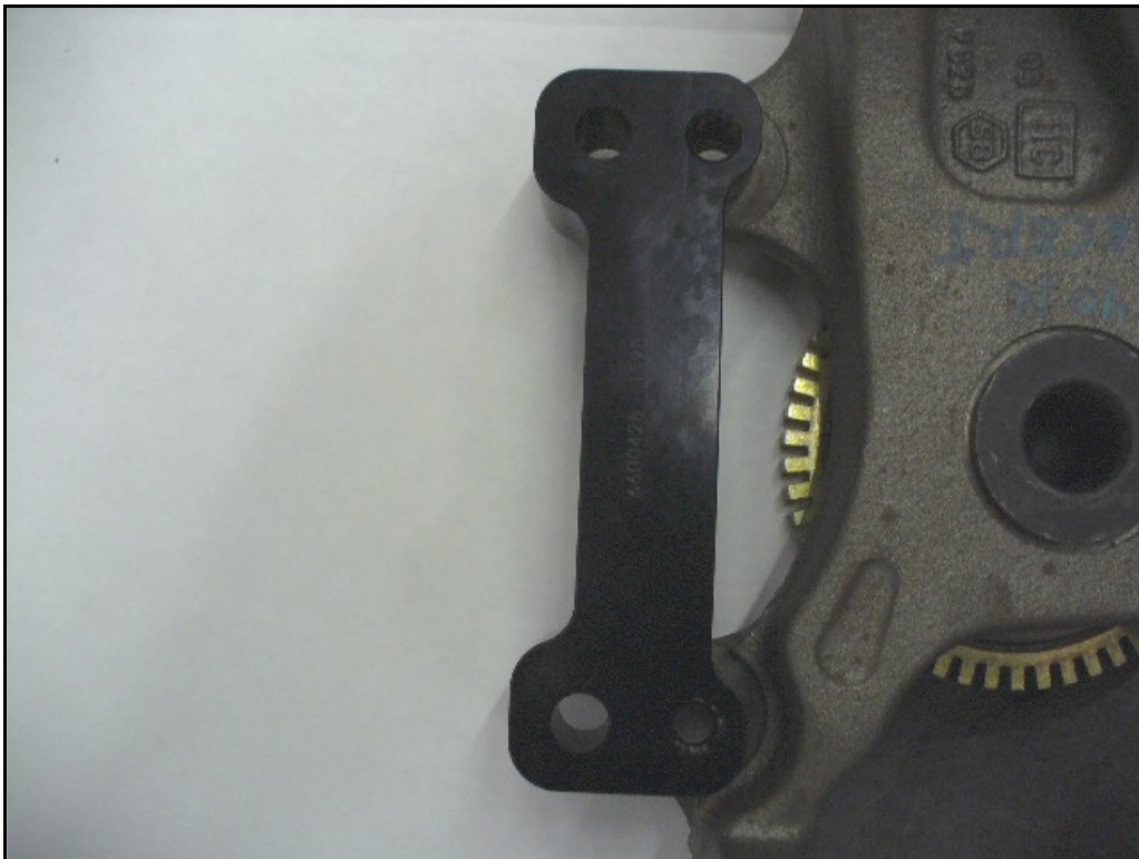
Bracket installed after caliper tabs trimmed.
