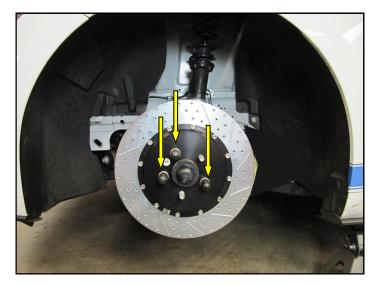
5. Install the Rotor onto the hub and secure it using three lug nuts and washers. NOTE: Rotors are directional and must be mounted at their corresponding location.
