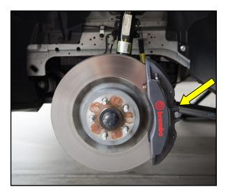
1. Separate the brake hose from the OEM caliper and plug or pinch the hose to prevent complete circuit drainage.
