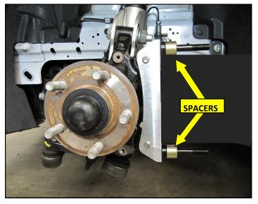
4. The Install the Radial Mount Bracket onto the outboard side of the spindle using the OEM bolts and the supplied 7/16" washers. Torque the bolts to 75 ft lbs. Slide the Spacers onto the Radial Mount studs as shown. NOTE: 14" rotors will use the .25 in Spacers and 15" Rotors will use the .75 in Spacers.
