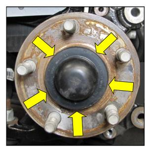
3. The BAER brake systems rotor has a very tight center bore by design. Remove any and all rust from the hub assembly to ensure the new components fit properly.
