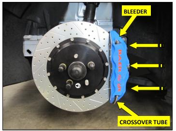
6. Slide the Caliper, with the Brake Pads installed and the bleeders on top, onto the Radial Mount Studs and secure it using the supplied 12 point Nuts and Washers. Torque the fasteners to 75 ft lbs.
