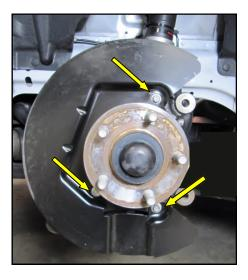
2. Remove the brake caliper from the vehicle and remove the three 6mm bolts holding the splash shield onto the spindle. The shield will not be used with the BAER brake system.
