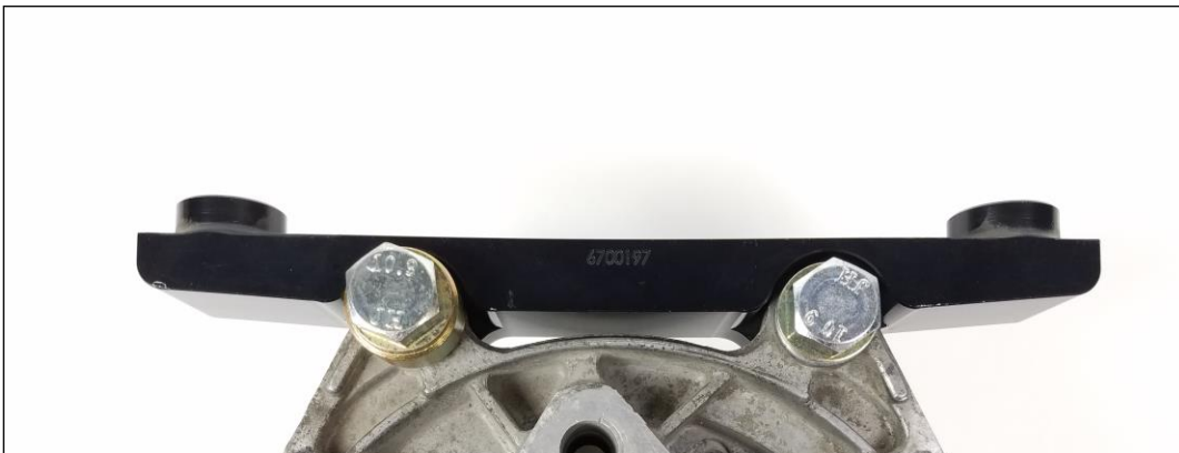
Figure 3: Bracket Installed with Spacer-Inboard View
