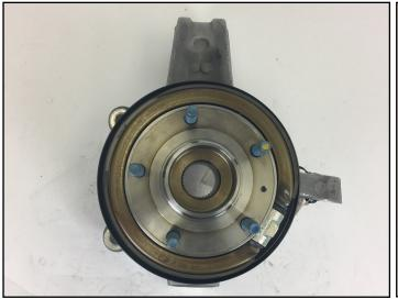
1. This installation begins at the point at which the factory brake caliper and rotor have been removed from the spindle and the brakes hardlines have been capped at the vehicle frame to prevent fluid from leaking. (Driver side rear shown)
