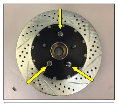
5. Make sure the hub snout is clear from debris to allow the rotor to sit flush against the hub face. Mount the rotor to the hub and temporarily secure it using 3 lug nuts and washers to prevent scratching the rotor hat.
