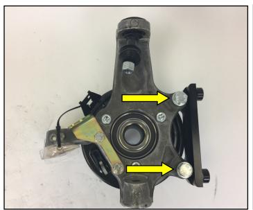
3. Inboard view of the Pro+ bracket installed.
