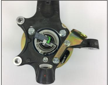
7. Outboard view of the park brake assembly installed. (Passenger side rear shown)
