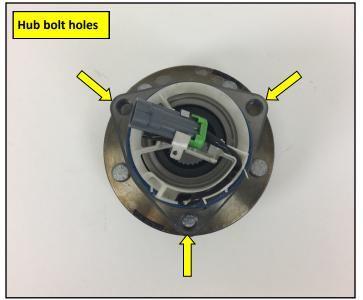
3. Set your hub face down on the studs. Make sure your ABS wire is facing in the correct direction.
