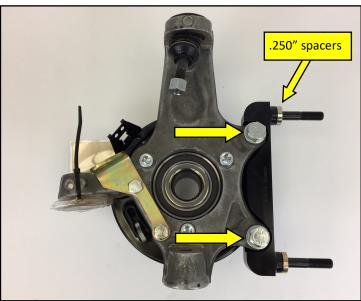
4. Inboard view of the Ext+ bracket installed. The 14" Ext+ system has .250" spacers on the ARP radial studs.
