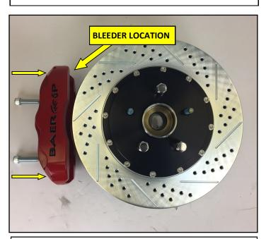
6. For Pro+ systems, install the correct side caliper with the bleeder pointing up and secure with the provided M12 socket heads. Make sure the caliper and rotor do not come in contact. Torque the socket heads to 85 ft-lbs.
