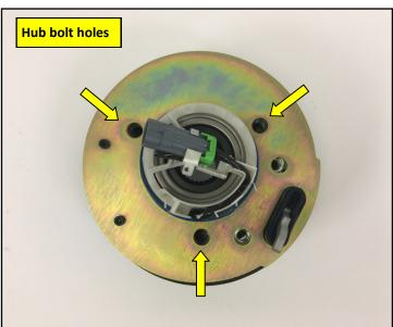
4. Now set the Baer parking brake assembly onto the hub. The shoe should fit around the hub flange. Line up the 3 hub bolt holes to the park brake plates holes.
