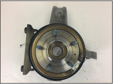
2. Make sure the bracket mounting surface is clear of debris. The bracket mounts to the outboard side of the knuckle with the flat side facing outboard. Secure the bracket to the spindle with the supplied M14 bolts and washers torqued to 110 ft-lbs.
