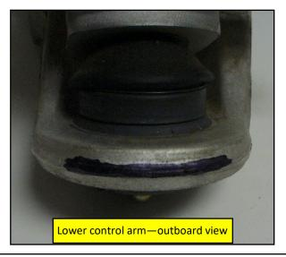
6. Check for adequate clearance between the rotor and the lower control arm just outboard of the ball joint. Due to production tolerances on the A-arm, our rotor may contact the casting lip at the nose. This will usually only happen when the suspension is loaded (normal ride height). A small lip is forged into the control arm and may require removal for clearance. Remove the lip about 0.750" from each side of center and recheck for clearance.
