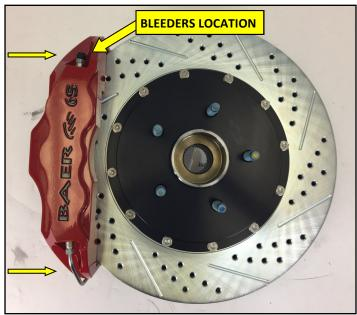
7. The Ext+ 6s caliper mounts onto the ARP studs installed into the bracket. Secure the caliper with the ARP washers and nuts. Check for clearance between the caliper and rotor and torque the nuts to 85 ft-lbs. to secure the caliper.
