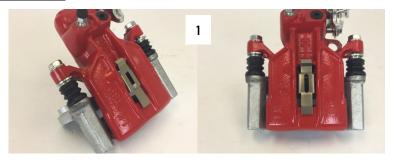
2. Install each pad abutment to the ears of the brake pad. The abutment should face away from the friction surface on the brake pad. There is a small tab that locks into place once the abutment is installed correctly.
