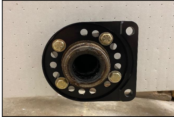
Figure 1: Base bracket installation (driver's side shown – bracket is engraved 6710133)
