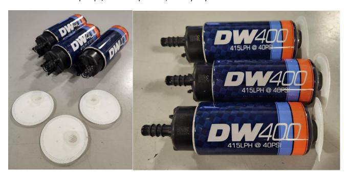
4 – Install the pumps into the bucket in the configuration shown below, two pumps at the back and one in the front. Double check that the filter socks did not pull the rubber check valves out of their holes.
