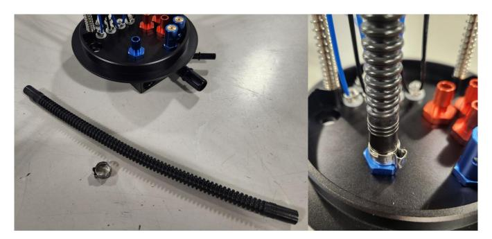
10 – You should have six convoluted tubes left, three longer 3/8" (10mm) and three shorter hoses. The shorter hoses are 3/8" (10mm) on one side and 5/16" (8mm) on the other. If your pumps have 5/16" outlet barbs use the shorter hoses, if you are using the DW400 pumps use the longer 3/8" (10mm) hoses. Attach the hoses to the three orange 3/8" (10mm) hose barbs on the X-series module tophat and secure with the included 13mm clamps.
