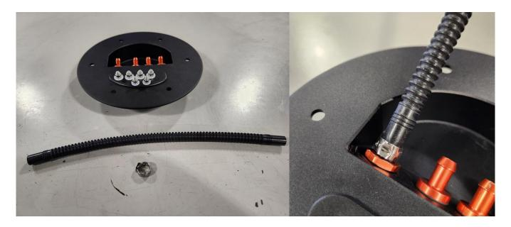
12 – Locate the three fuel pump pigtails, and the six 16-14awg ring terminals. Strip and crimp the ring terminals to the pigtails. Leaving the pigtails at their current length will help with installation, shorten them at your own discretion.
