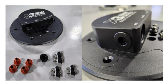
8 – Install the four orange 6ORB hose barb fittings on the underside of the tophat assembly.
