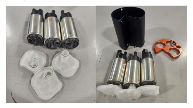
4 – Slide the pumps into the bucket as shown below. Install the orange pump holder on top of the pumps and install the three screws into the pump holder, the shorter screw goes in the location behind the fuel level sensor.
