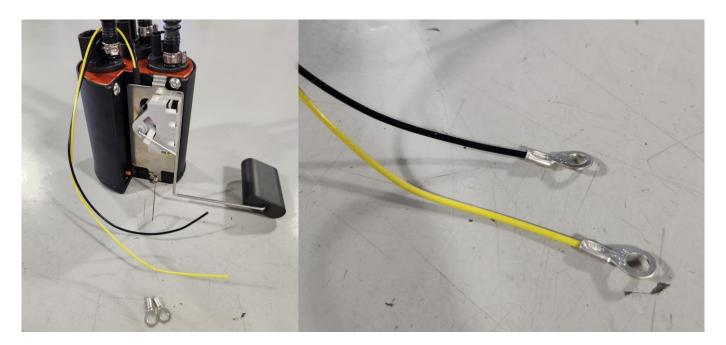
14 – Attach the fuel pump pigtails to the wiring terminals. One pump should be attached to the "Stage 1" terminals and the remaining two pumps to the "Stage2" terminals.
