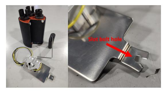
6 – There is a notch in the X-series surge bucket designed for the level sensor. Slip the top edge of the level sensor between the orange pump holder and surge bucket at this notch and secure the level sensor and black level sensor ground wire with the included 2.5mm hex M3 socket head bolt.
