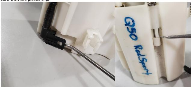
10 – Install the pump power adapter harness onto the DW pump and the top hat, and re attach the fuel level sending unit and fuel temp/low level sensor, and plug the wiring for each back in.
