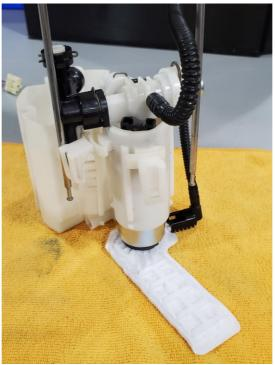
8 – Install the pump and center section back into the bucket. Fold the filter sock up along side the pump for easier installation. Once the pump is seated against the bottom of the bucket, press down on the locking tabs and re-latch them over the bucket, these will stretch a small amount to make up the difference in fuel pump heights.
