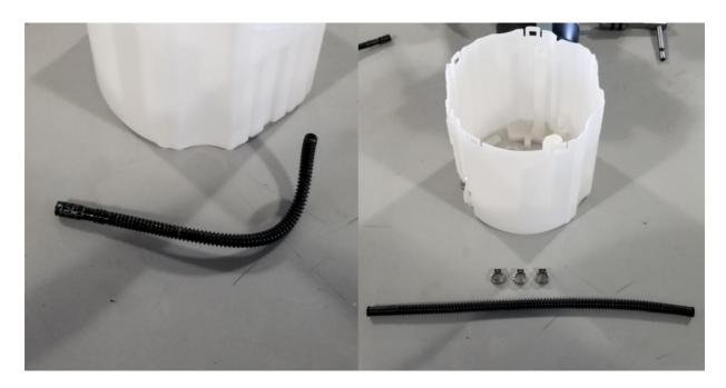
16 - Push the hose onto the bard inside the bucket and then slide a hose clamp down. You can use a pair of side cutters to pinch the clamp. Marked in the  $2^{nd}$  picture is where we need to pinch.
