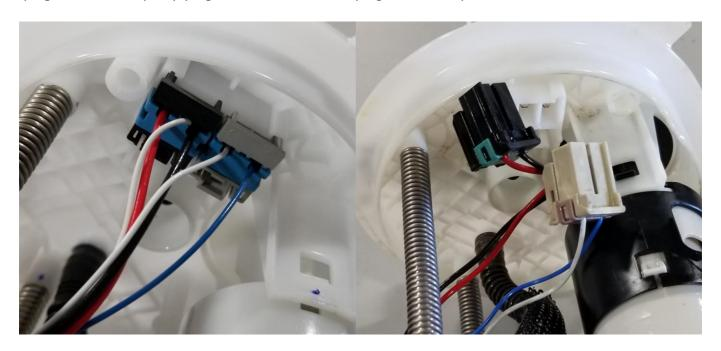
4 – Now you can fish out the fuel level sender and set this to the side as it will need to be reinstalled later.
