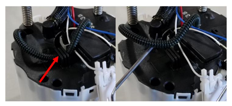
2 – Depress the 2 tabs on the fuel level sender to un-latch it from the module then pull up.
