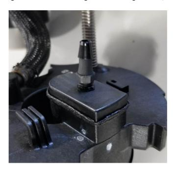
14 - We need to replace the venturi hose. Use a razor blade to cut the hose shown in the  $2^{nd}$  picture. Take care to not damage the barbs under the hose.
