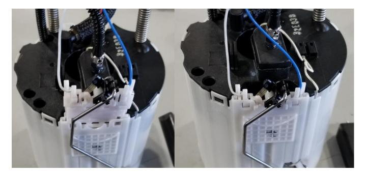
26 – Plug in the fuel level sender harness into the top hat.
