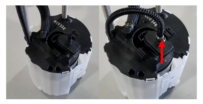
22 – Plug in the fuel pump harness into the pump. Slot the small static ground back into the top of the filter assembly like it was before.
