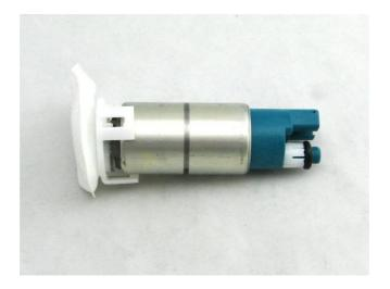
4 (2010-2012) – prep the supplied pre-filter for use by separating the PRV retainer from the pre-filter. The clips are orientated slightly different, this will make the installation easier. Install the retainer onto the OE PRV first.
