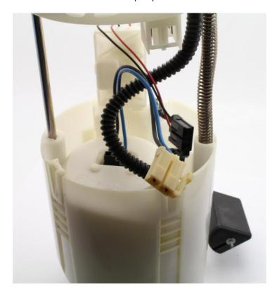
2 – disconnect the venturi jet and separate the fuel level sender from the assembly
