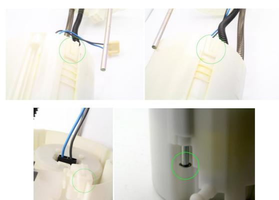
4 – unclip the fuel sock form the center assembly and pull the fuel pump out
