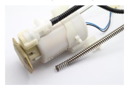
7 – install center assembly into bucket and reconnect the fuel level sender
