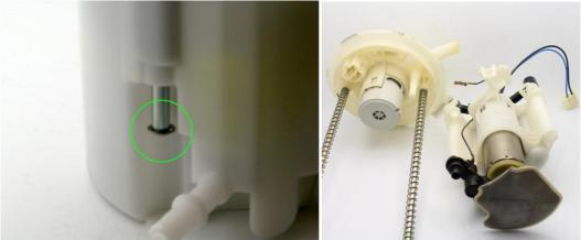
4 – remove the fuel pump from the center section by using 2 flat-head screwdrivers to open the retaining tabs (green)
