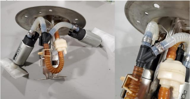
10 – Plug the factory connectors back into the pumps, due to the special notch that's been added to the Deatschwerks pumps the factory connectors plug directly into the new pumps. Re-install the factory band strap onto to the module, hook the end through the eyelet on the module and secure with the OEM 9/32" screw.
