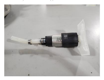
8 – The supplied convoluted fuel hose has different sized openings at each end. The smaller end is designed for the Deatschwerks fuel pump, slip it on and secure it with one of the supplied hose clamps, repeat this on both fuel pumps.
