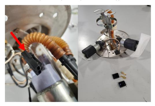
4 – Using a pick or small flat blade screwdriver depress the locking tab and remove the factory pins from the special notched connector, make sure to keep the wires in the same spots or the pumps will spin backwards.
